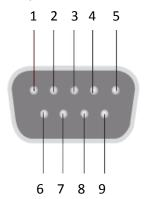
The pinouts for the USB to Serial converter cable (P/N 88049-03) are:
